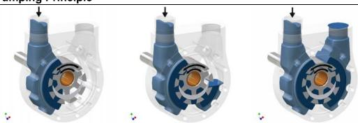
Tuthill MG Series pumps employ the internal gear pumping principle. There are only two moving parts. Pumping action is based on a rotor, idler gear and crescent-shaped partition cast integral with the cover.
