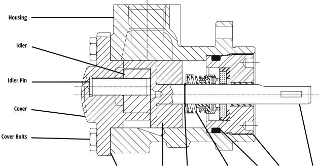
Cover Gasket Housing Bushing Retaining Ring Seal Assembly O-Ring Housing Plug Rotor
