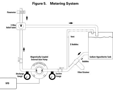
Valves designed with vent option (hole) for sodium hypochlorite use are recommended to prevent off gassing.
