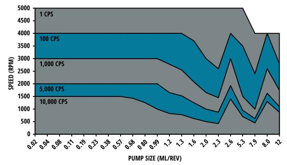
Note: Recommended pump speed is 3600 - 700 RPM.
