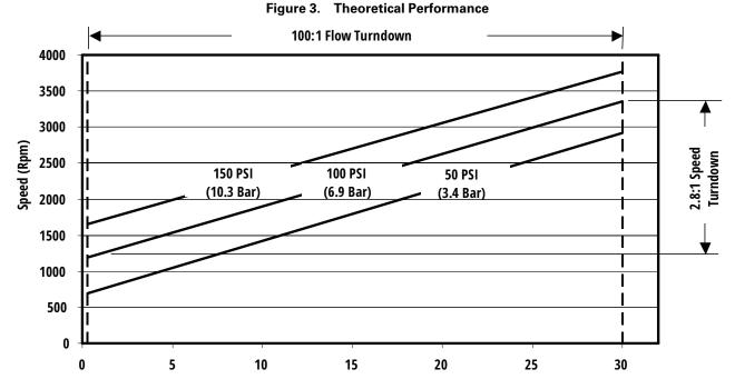
**Note:** For this application, the 0.68 ml/rev displacement pump at 100 psi (6.9Bar) differential pressure, achieves a 100:1 flow turn down with a 2.8:1 speed turn down.
