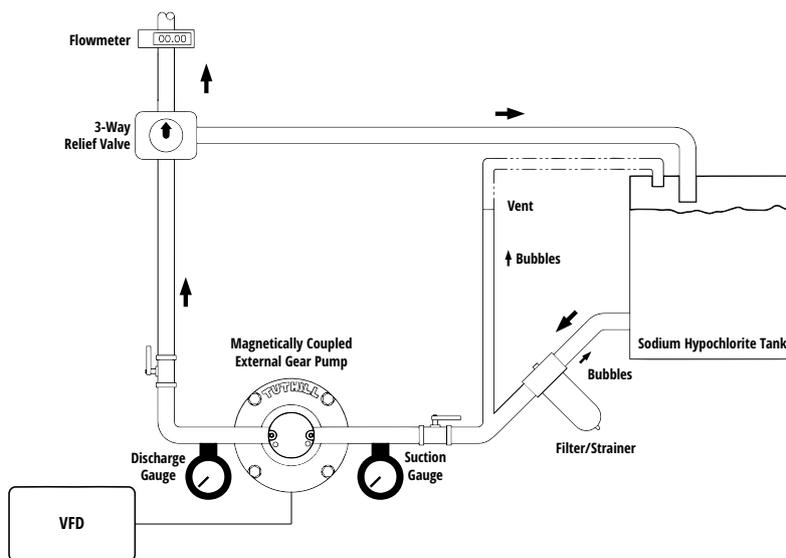
Valves designed with vent option (hole) for sodium hypochlorite use are recommended to prevent off gassing.
