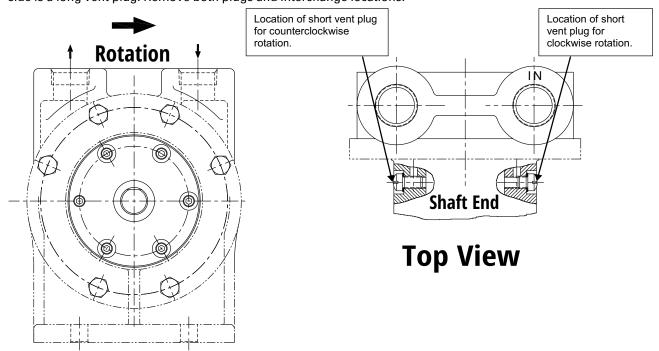
If outfitted with an internal relief valve (model CK1BV), the rotation cannot be changed in the field unless the cover/valve assembly is also replaced. To change the location of the suction port on pumps supplied with Ingersoll Rand's unique automatic reversing feature (model RCK1B), the following must be done in addition to the steps above.
