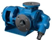
Standard gall-resistant, Nitronic 60 rotor head & idler gear Differential pressures to 150 PSI (10.3 bar) Temperatures to 500 °F (260 °C) Viscosities to 1,000,000 SSU (220,000 cSt) Max differential pressure to 100 PSI if fluid is < 100 SSU
